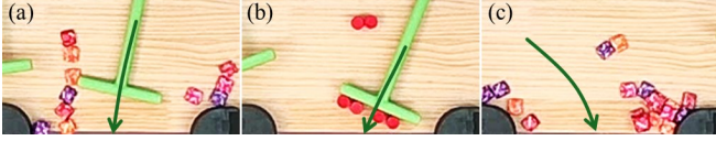
Fig. 7. Failure cases: (a) Redundant pushing path selected by the task planner; (b)-(c) Premature pushing resulting in outliers.
