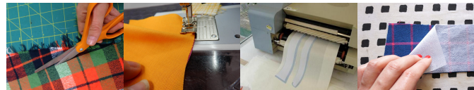
Fig. 1. Fabric alignment is a fundamental task essential to various garment manufacturing processes, including (from left to right) fabric cutting, sewing, fusing, and pattern matching.
