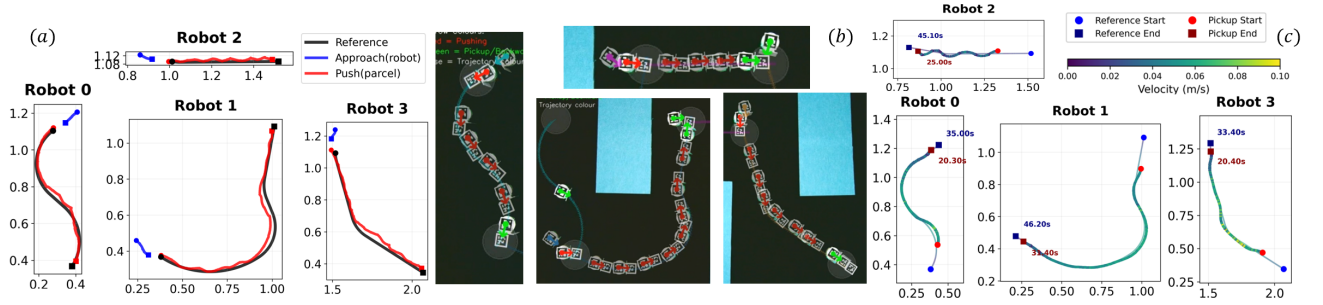
Fig. 13. The experiments result of Fig. 9 case of pushing parcel 1: (a) The pushing trajectory; (b) The snapshots of the pushing process; (c) The pickup trajectories, color-coded by velocity.
