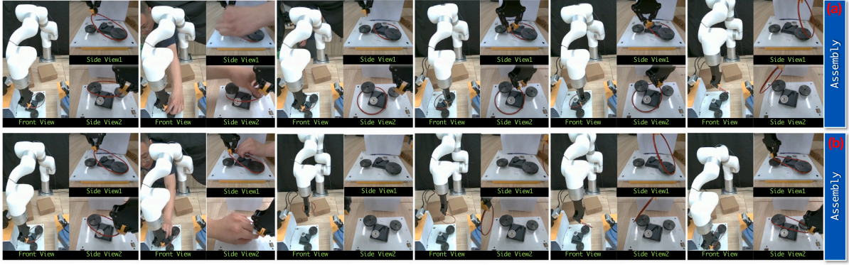
Fig. 8. Experimental results of error recovery in assembly tasks for the round belt drive system using our LLM+DP3+Query approach. The figure illustrates cases where, following external disturbances that remove the belt from the gripper, the system successfully recovers and completes the assembly task.
