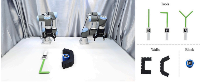
Fig. 1. Tool-Object manipulation in a dual-arm robotics system with environmental constraints using the non-prehensile approach.
