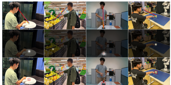
Fig. 7. Some estimation results during the testing process for location L programming. The first row illustrates the estimated gaze/hand-pointing direction alongside the ground truth gaze/hand-pointing direction. The second row shows the heatmaps generated from the first row. The third row shows the target estimated based on the heatmap.
