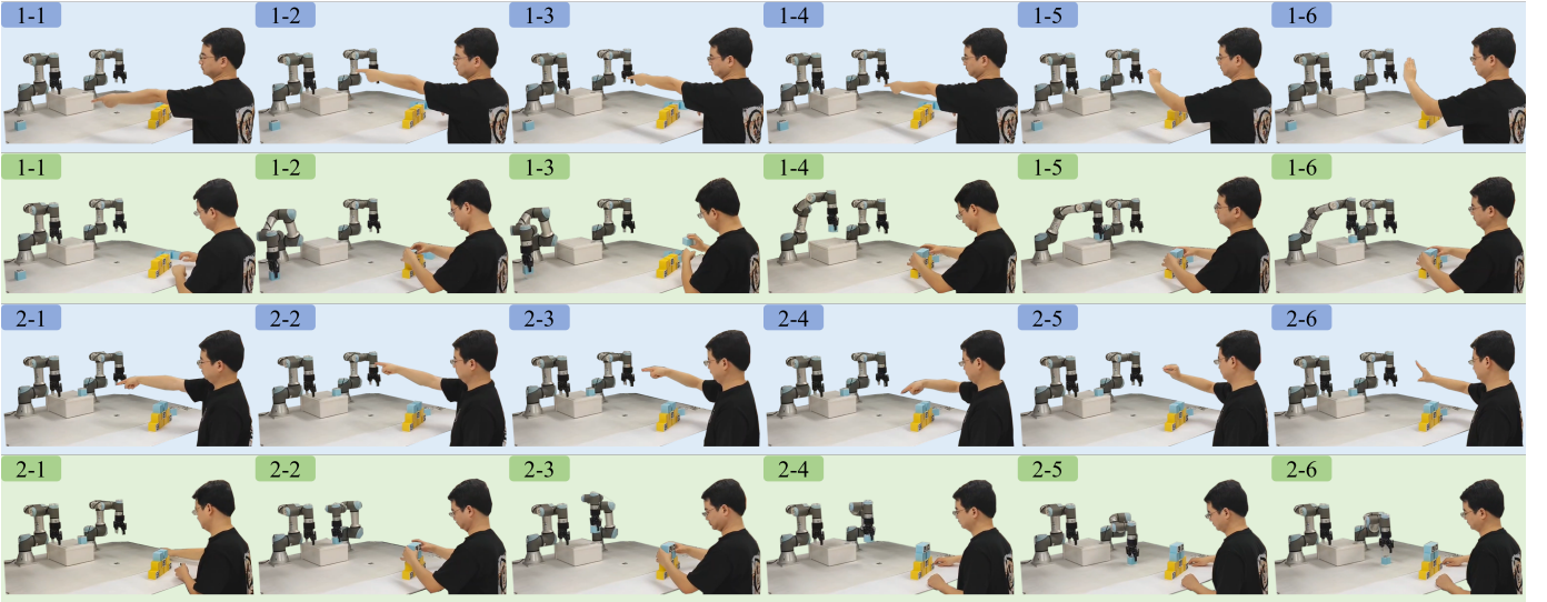
Fig. 11. Robot programming procedures for two subtasks of the "Playing the Building Blocks Together" task. For each subtask, the blue blocks denote the human programming stage, in which the user specifies the task elements \{L, M, O\} through body language, whereas the green blocks denote the subsequent robot execution stage. The numbered snapshots (e.g., 2-1) indicate the temporal progression of the task: the first digit denotes the subtask index, while the second digit denotes the action order of the end-user or the robot within that subtask. The sequence further shows that robot execution begins only after the corresponding human programming process is completed.
