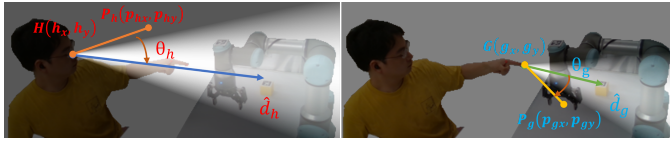
Fig. 5. A description of the methodology for creating a gaze/hand-pointing direction field. The blue line represents the direction of the individual's gaze, while the green line indicates the direction of the hand-pointing gesture.
