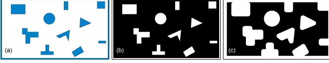
Fig. 4. Example map for path planning: (a) the original map; (b) the occupancy map; (c) the inflated occupancy map.
