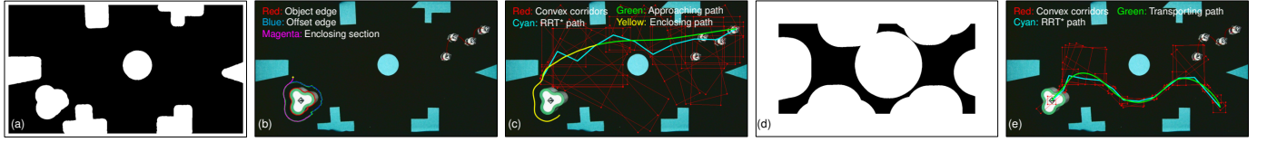
Fig. 15. Path planning for transporting a single object: (a) The inflated occupancy map for approaching and enclosing steps; (b) The object enclosing section; (c) The path planning results for approaching and enclosing steps; (d) The inflated occupancy map for the transporting step; (e) The path planning results for the transporting step.
